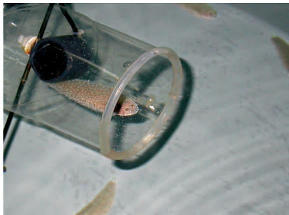
Detail of the infrared sensor to activate the self-demand feeders.
